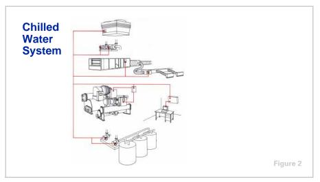
Water chillers are used in a variety of air conditioning and process cooling applications. They are used to make cold water that can be transported throughout a facility using pumps and pipes. This cold water can be passed through the tubes of coils in order to cool the air in an air conditioning application or it can provide cooling for a manufacturing or industrial process.
